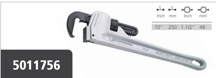
5011756 Aluminium Pipe Wrench 10" One-handed pipe wrench. Features similar to HEAVY DUTY. Weight savings of approx. 40%: extremely light, high strength aluminium alloy. Wearing parts replaceable: hook and heel jaw can be purchased separately.
