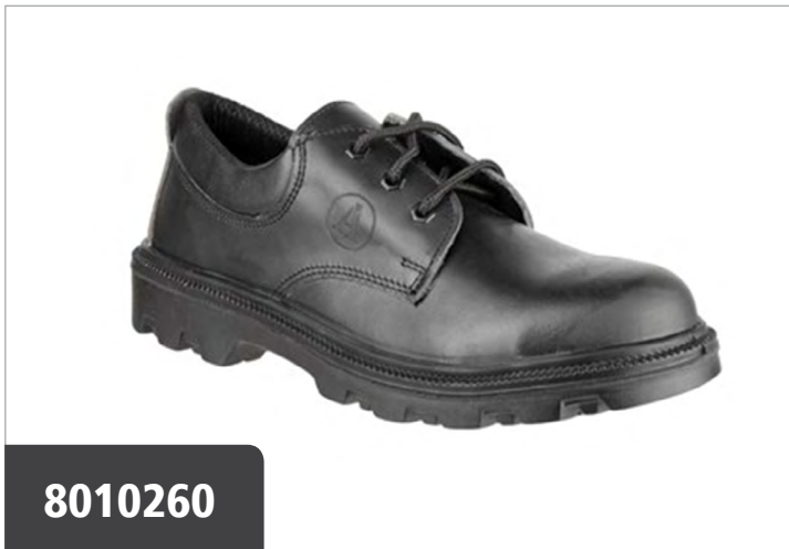
8010260 S3 Black Lace-Up Safety Shoe Midsole. Antistatic. Water Resistant. Toe Protection. Resistance to high heat. Heel energy absorption. Rubber / PU sole. SRC Slip Resistance. Sizes: 6 - 12 Category: S3-HRO. Slip Resistance: SRC Standard: EN ISO 20345:2011
