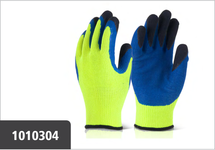
1010304 Latex Thermo-Star Fully Dipped Glove Special reinforcement on fingertips offers added protection and can extend the life of the gloves. Mixed fibre heavyweight knitted liner with Latex coated to palm area. Double dip to fingers. Vented back. Highly visible fleece liner. Ideal for refrigeration, coldstore, general use and winter conditions. Thick latex coating for durability and grip. Size: 8 - 11 Standard: EN388 2.2.4.1. EN511 1.4.X
